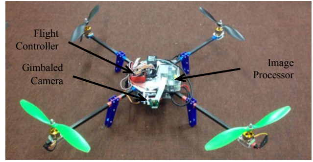
Fig. 2. Quadcopter UAV and control system hardware.
