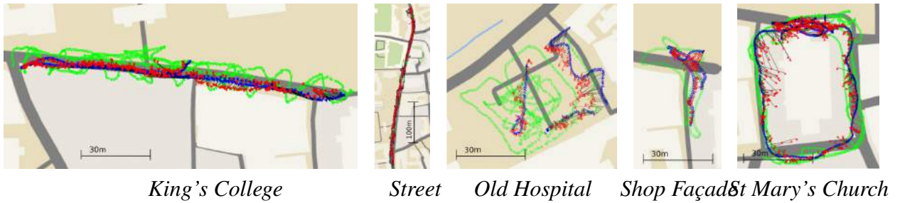
Fig. 3.5 Map of dataset showing training frames (green), testing frames (blue) and their predicted camera pose (red). The testing sequences are distinct trajectories from the training sequences and each scene covers a very large spatial extent.
