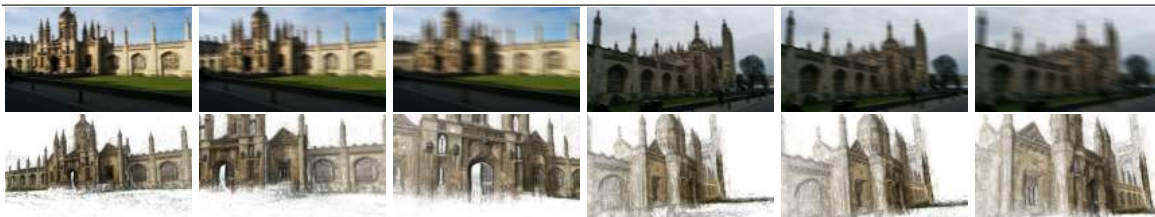
(a) Relocalisation with increasing levels of motion blur. The system is able to recognize the pose as high level features such as the contour outline still exist. Blurring the landmark increases apparent contour size and the system believes it is closer.
