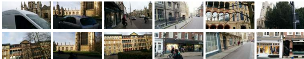
Fig. 3.22 Images with the largest uncertainty values and largest localisation errors. All of these images contain one of the following situations that cause difficult and uncertain localisation: strong occlusion from vehicles, pedestrians or other objects, motion blur, are taken from an area at the edge of the scene or are distant from a training example.
