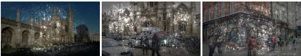
Fig. 3.10 Saliency maps. This figure shows the saliency map superimposed on the input image. The saliency maps suggest that the convolutional neural network exploits not only distinctive point features (à la SIFT), but also large textureless patches, which can be as informative, if not more so, to the pose. This, combined with a tendency to disregard dynamic objects such as pedestrians, enables it to perform well under challenging circumstances. (Best viewed electronically.)
