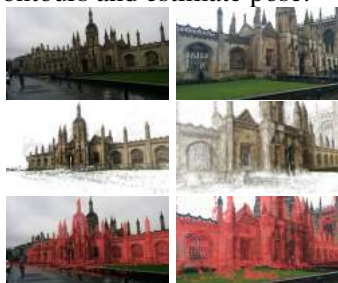
(c) Relocalisation with different weather conditions. PoseNet is able to effectively estimate pose in fog and rain.
