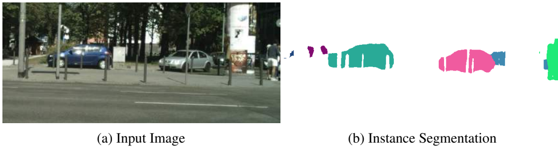
Fig. 2.19 This example shows two cars which are occluded by trees and lampposts, making the instance segmentation challenging. Our instance segmentation method can handle occlusions effectively. We can correctly handle segmentation masks which are split by occlusion, yet part of the same instance, by incorporating semantics and geometry.
