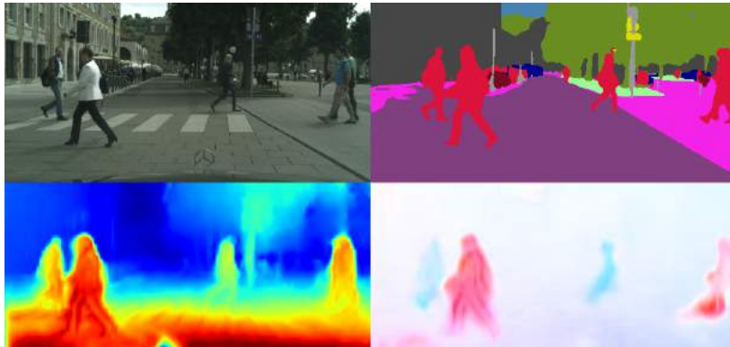
Fig. 5.1 Video scene understanding. Our model jointly learns to estimate scene motion (bottom right), depth (bottom left) and semantic segmentation (top right), in addition to estimating ego-motion over video input. We learn semantics with supervised learning and are able to learn geometry and motion using self-supervised learning, without labelled training data.
