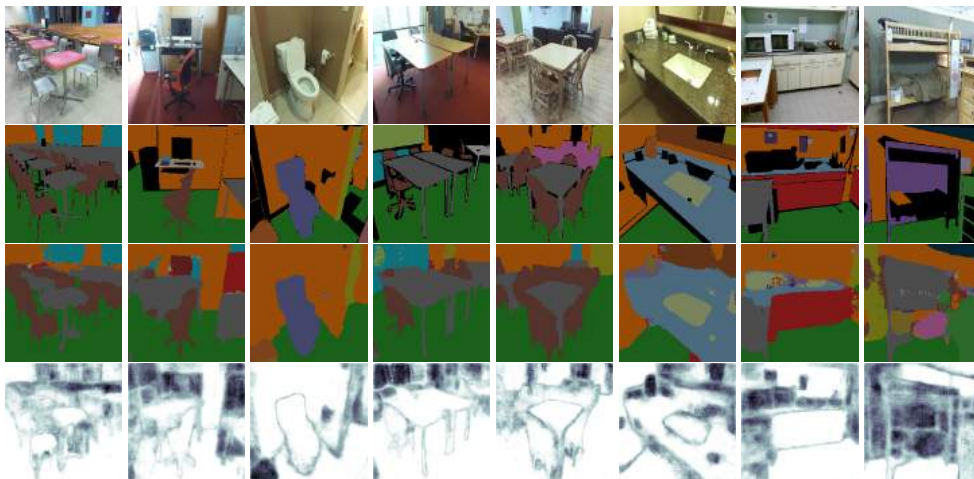
Fig. 2.9 Bayesian SegNet results on the SUN RGB-D dataset. From top: input image, ground truth, Bayesian SegNet's segmentation prediction, and overall model uncertainty averaged across all classes.
