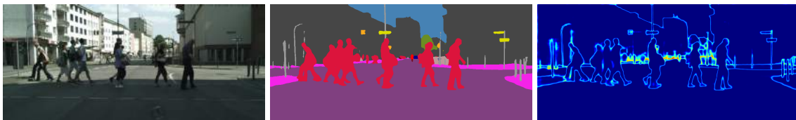
(c) Uncertainty — understanding the prediction’s confidence and what the model does not know. From left: input image, semantic segmentation, model uncertainty (where blue represents certain and more red colours are uncertain predictions). The model exhibits increased uncertainty in distance objects and around object boundaries.
